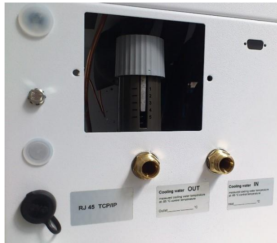
Figure 2 Open the cover of the cooling water flow regulator
