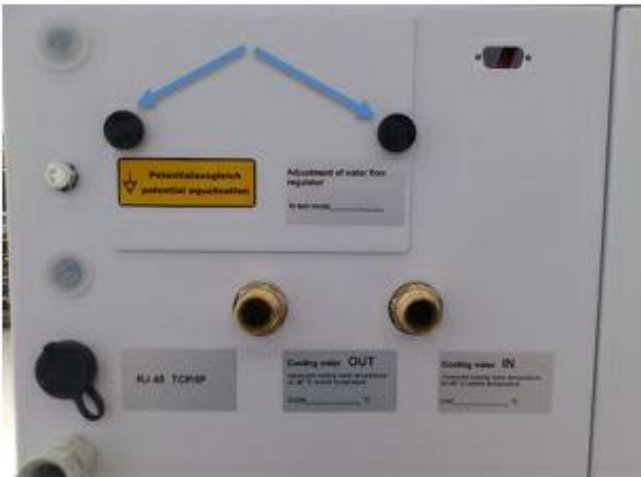
Figure 1 Unscrew the knurled screw
