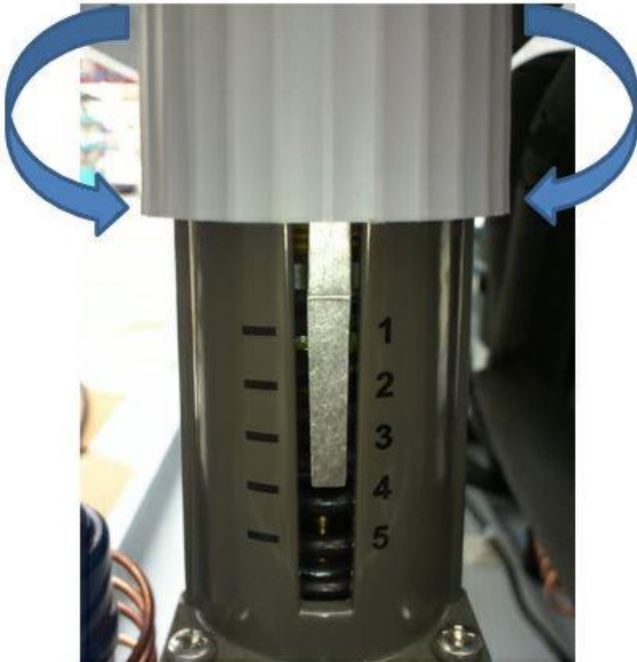
Figure 3 Turn the adjustment wheel towards the 1 on the scale to increase the cooling water flow; turn it towards the 5 on the scale to reduce the quantity of cooling water.
